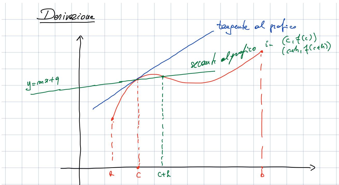
$$\frac{y - f(c)}{f(c+h) - f(c)} = \frac{x - c}{(c+h) - c} \Rightarrow m = \underbrace{\frac{f(c+h) - f(c)}{h}}_{\text{rapporto incrementale}}$$
